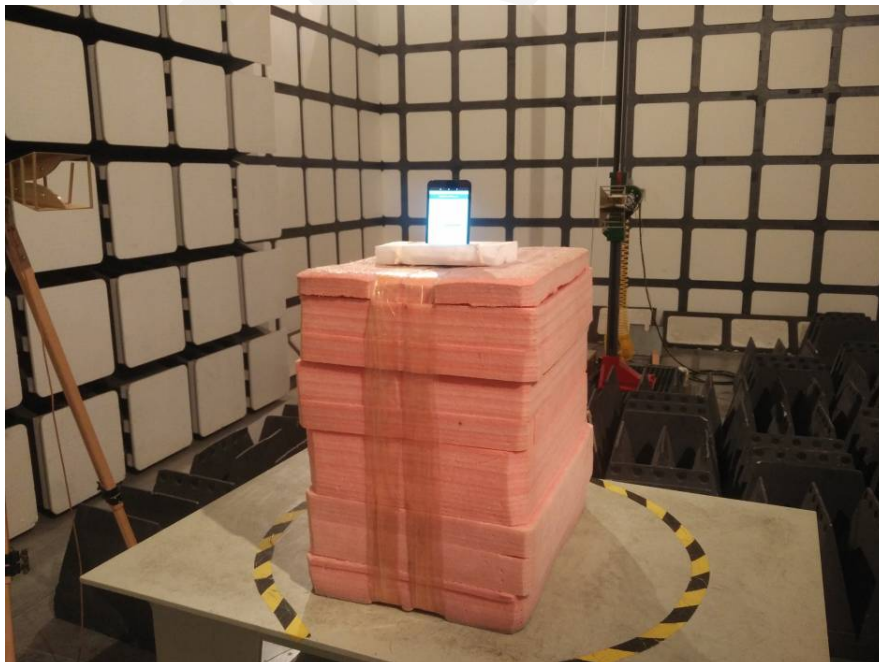
Radiated Spurious Emissions Test View (Above 1GHz)
