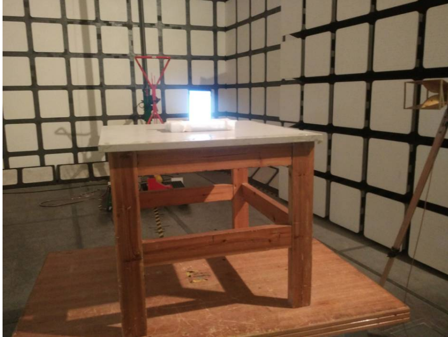
Radiated Spurious Emissions Test View (Below 1GHz)
