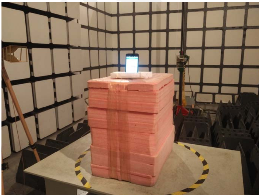
Radiated Spurious Emissions Test View (Above 1GHz)
