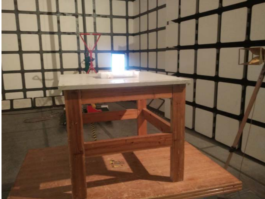
Radiated Spurious Emissions Test View (Above 1GHz)
