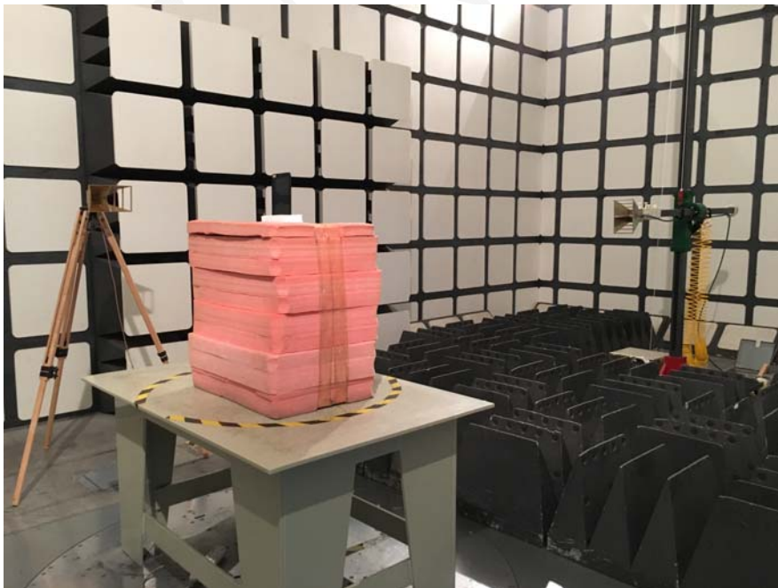
Radiated Spurious Emissions Test View (Above 1GHz)
