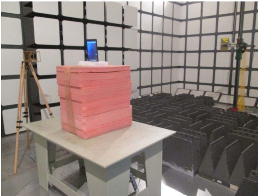
Radiated Emissions View (Above 1 GHz)
