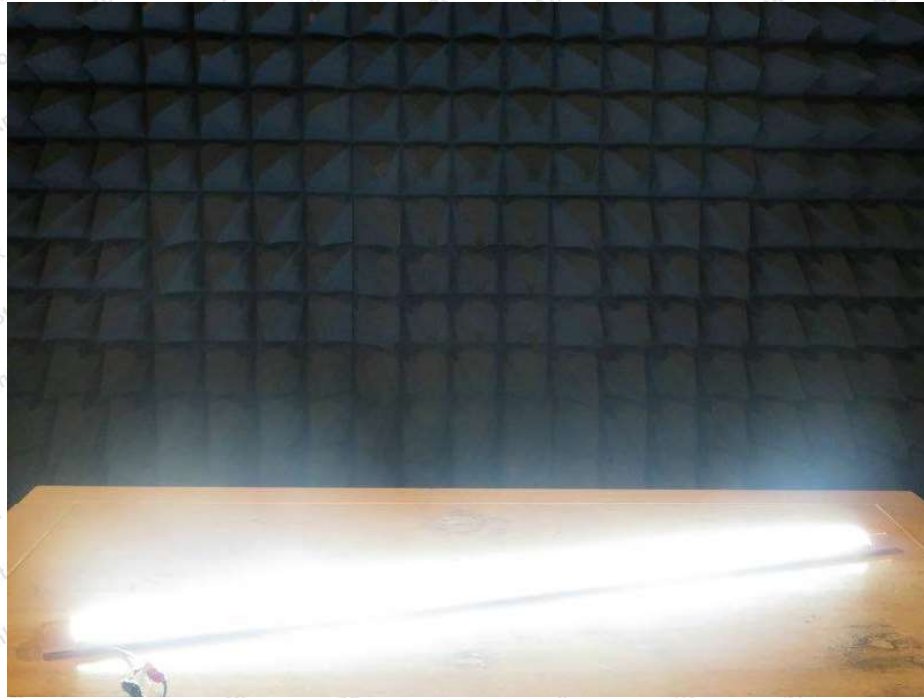
Photo of RF Field Strength susceptibility Test
