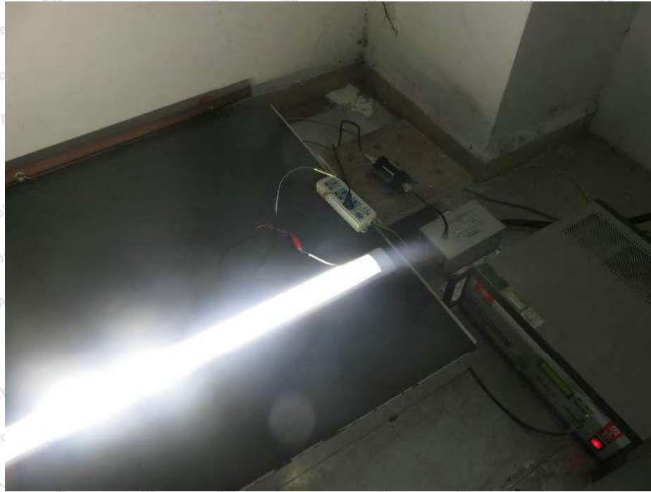
Photo of Injected currents susceptibility Test
