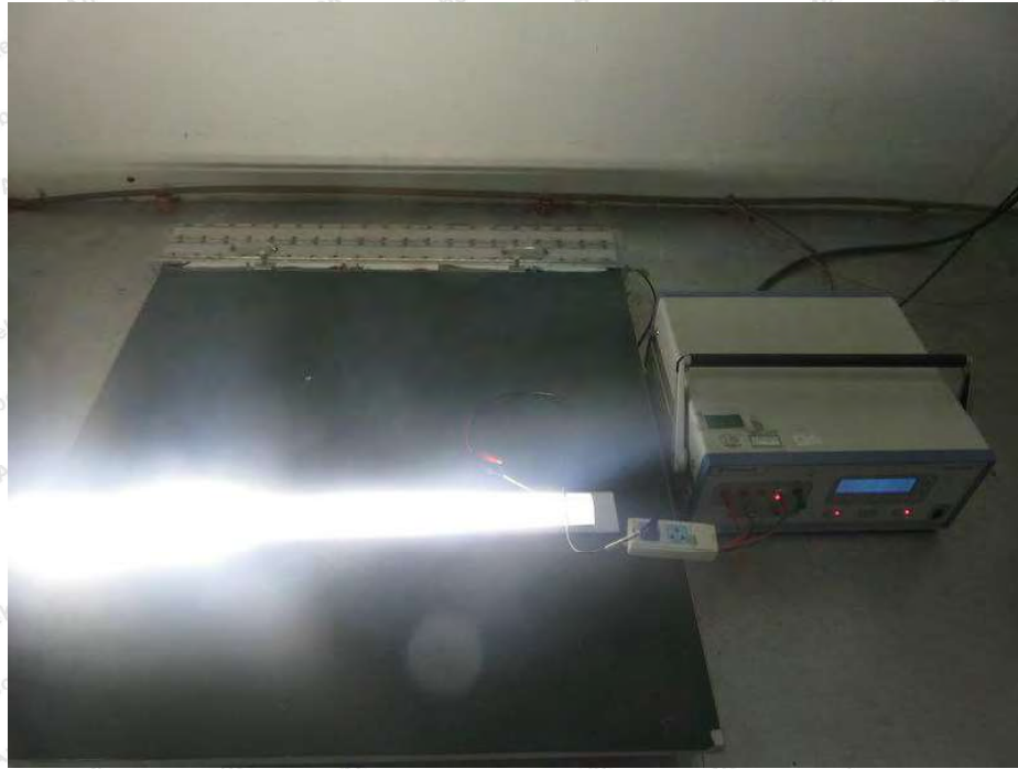
Photo of Electrical Fast Transient/Burst Immunity Test
