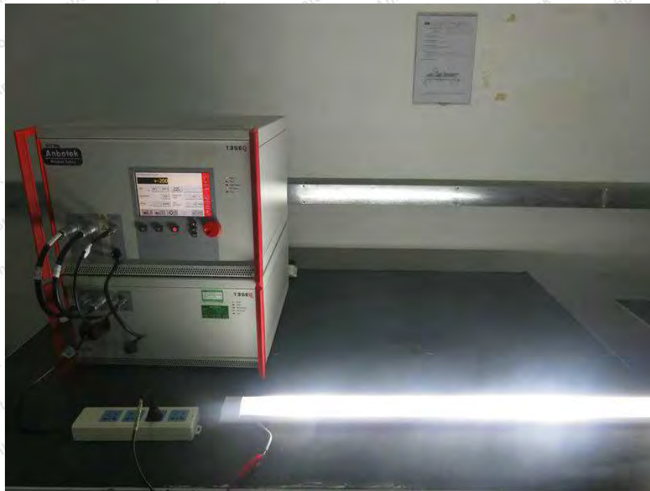
Photo of Surge Immunity Test
