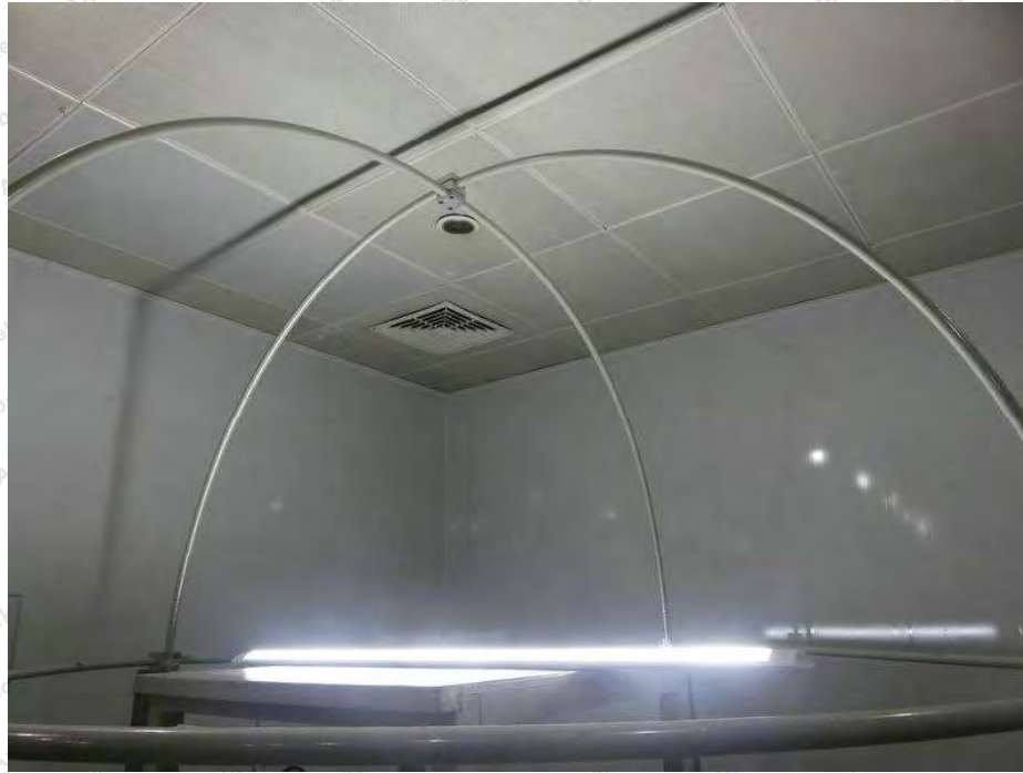
Photo of Magnetic Radiated Emission Test
