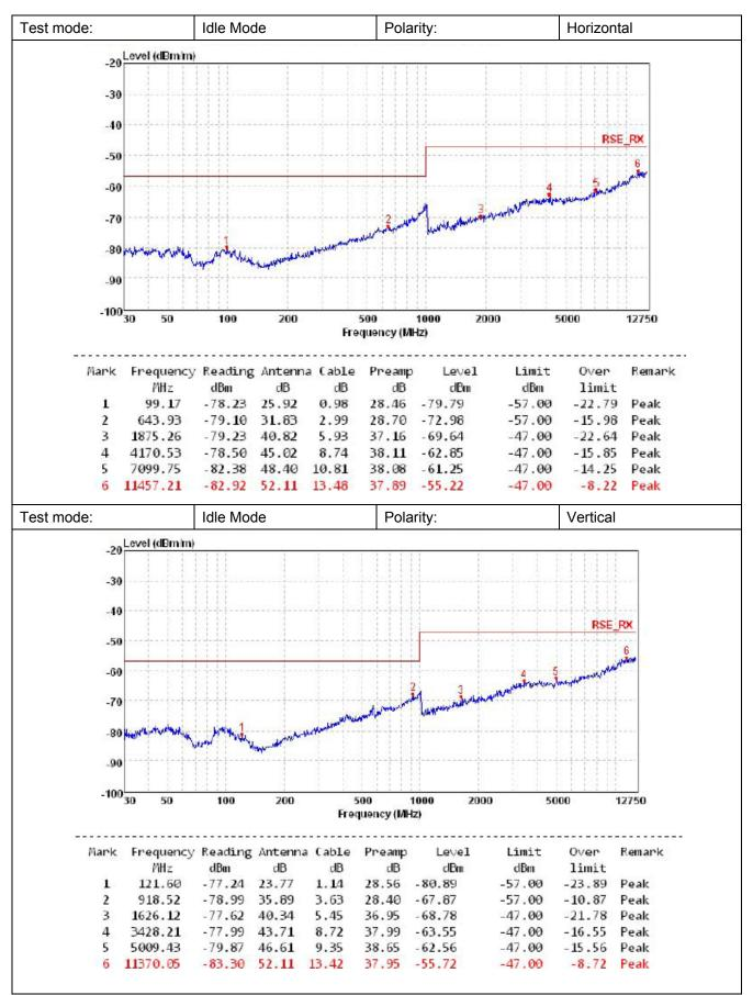
Note: The radiated spurious are performed the each test mode(WCDMA,HSDPA,HSUPA), the datum recorded is the worst case for all the mode at WCDMA mode.
